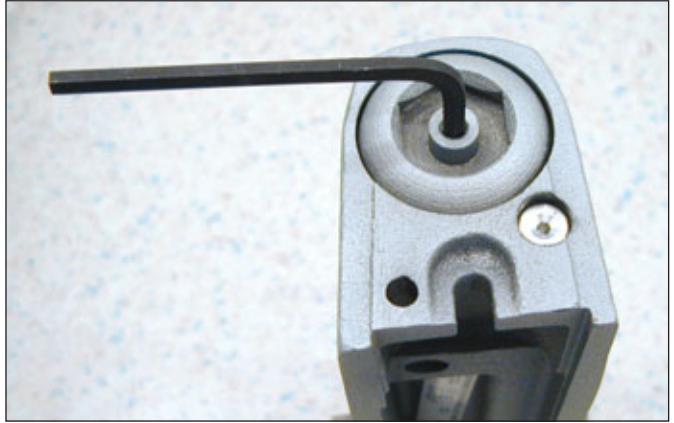
16. The spring can be adjusted from a #1 to a #5 power.
